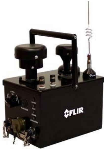
Figure 1 - FIDO B2 IBAC Bio-aerosol Detector
