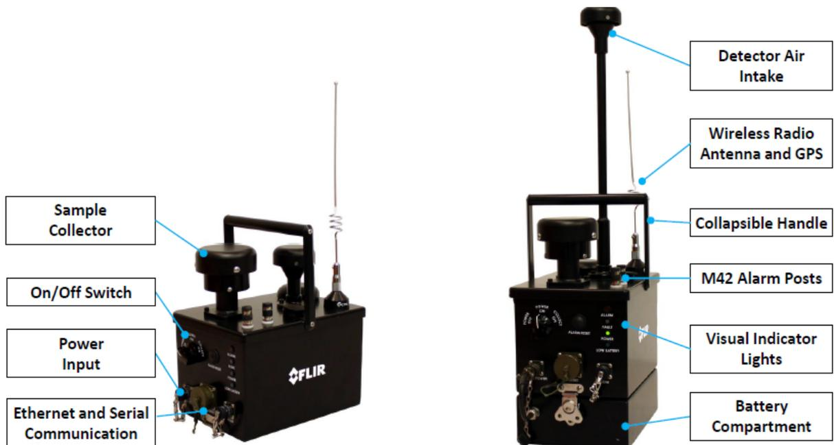
Figure 2 - FIDO B2 IBAC Bio-aerosol Detector Parts and Componentes
