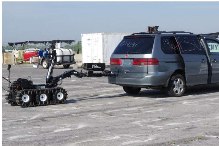
Figure 2 – The Knight robot with HAZPROBE preparing to drill into suspect vehicle
