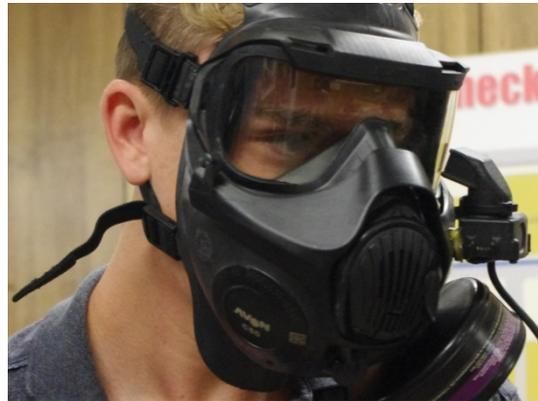
**Figure 2 – Photograph of Situational Head Up Display Attached to Avon's M53 Mask**
