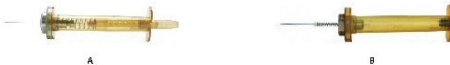
Figure 2– Samples can be collected and introduced to the unit via PerkinElmer’s SPME (A) or Custodian-NT (B) syringes.
