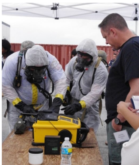
Figure 3 - First Responders Preparing to Inject a Sample into the Tridion-9 during the OpEx Event.
