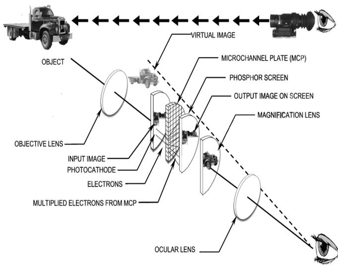
Figure 2: Gen 2 and Gen 3 Tube Components
