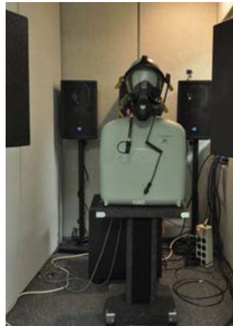
An example setup used for conducting audio quality testing.
