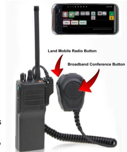
Turtle Command™ Field User Hardware: The Turtle Command™ shoulder microphone and Turtle Alert™ smart device application allow the end user to leverage existing LMR and commercial broadband networks
