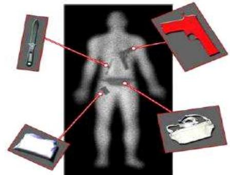
**Passive Millimeter Wave Image**
