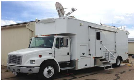
**Figure 4-1. COLT System with Satellite Backhaul**
