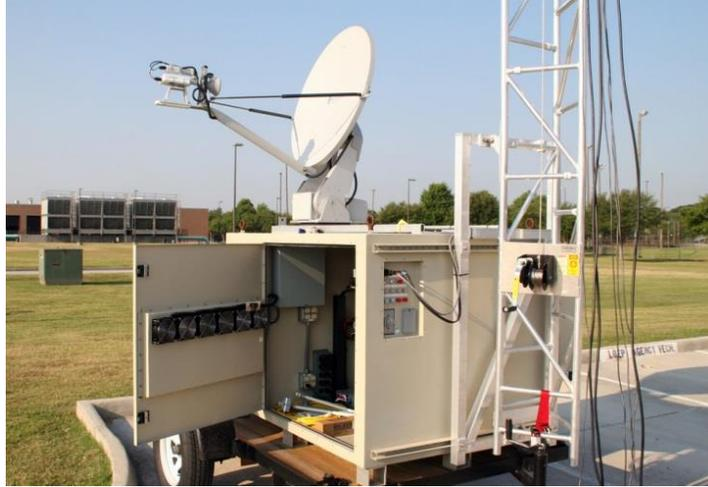
**Figure 3-1. COW System with Both Satellite and Tower Antenna Backhaul**
