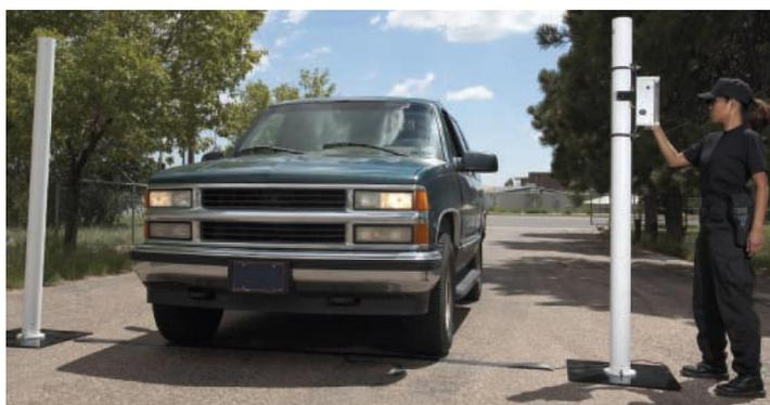
**Figure 2-1. PRPM in use as a vehicle monitor**
