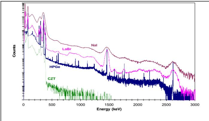
Figure 1. Comparison of Ba-133 calibration source gamma-ray spectra for CZT, HPGe, LaBr<sub>3</sub>(Ce) and NaI(Tl) crystal detectors. Note that the best resolution is obtained with HPGe, followed by LaBr<sub>3</sub>(Ce) and NaI(Tl). Note also that CZT has low sensitivity for gamma ray energies above 400 keV.
