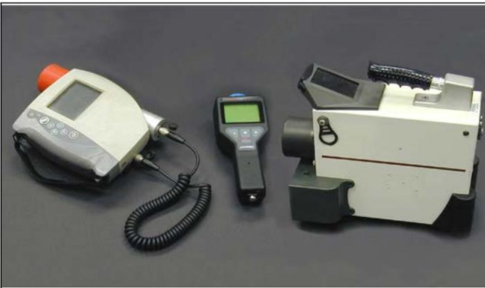
Figure 2. Typical handheld RIID detection systems; left to right: LaBr<sub>3</sub>(Ce), NaI(Tl), and HPGe.
