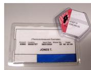
Thermoluminescence dosimeters (TLDs) and optically stimulated luminescence (OSL) dosimeters contain materials that trap electrons released during radiation exposure which can later be freed by stimulation with heat (TLD) or light (OSL). This stimulation is done in a processing laboratory and the resulting light emission provides a measure of the radiation dose received. TLDs and OSL dosimeters are widely used in worker radiation safety programs.
