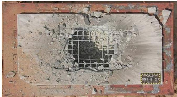
Damage sustained to a reinforced concrete slab during testing. (Photo courtesy of USACE-ERDC)
