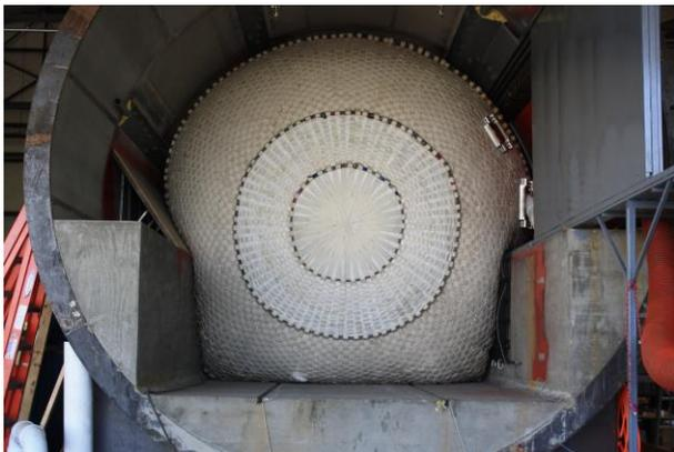
The tunnel plug conforms to the shape of a subway tunnel to stop flooding.
