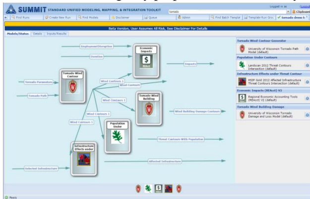
Figure 2. Linking of models in SHERPA templates
