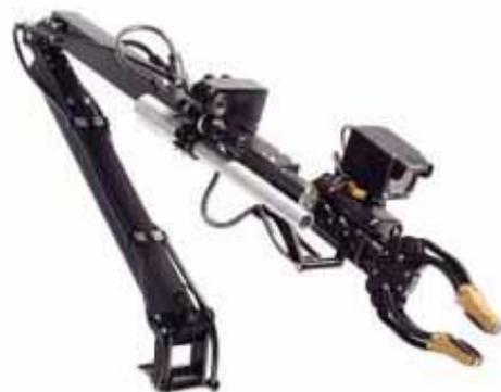
**Figure 2-3. Articulating Arm Equipped with a Gripper and Camera**
