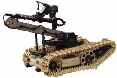
The robot is powered by one BB-2590/U rechargeable lithium-ion battery. The CCU is powered by one internal rechargeable lithium-ion battery. The robot is environmentally sealed and is chemical-biohazard washdown safe. Accessories and attachments available for an additional cost include:
