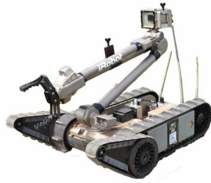
One to four BB-2590/U rechargeable lithium-ion batteries power the robot. The CCU is powered by the laptop that uses a proprietary rechargeable battery. The robot is environmentally sealed and is chemical-biohazard washdown safe. Accessories and attachments available for an additional cost include:
