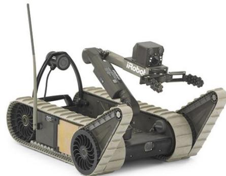
One or two BB-2590/U rechargeable lithium-ion batteries power the robot. The CCU is powered by one BB-2590/U rechargeable lithium-ion battery. The robot is environmentally sealed and is chemical-biohazard washdown safe. Accessories and attachments available for an additional cost include:
