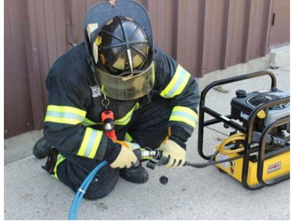
**Figure 3 – Evaluator setting up the hydraulic extrication device**
