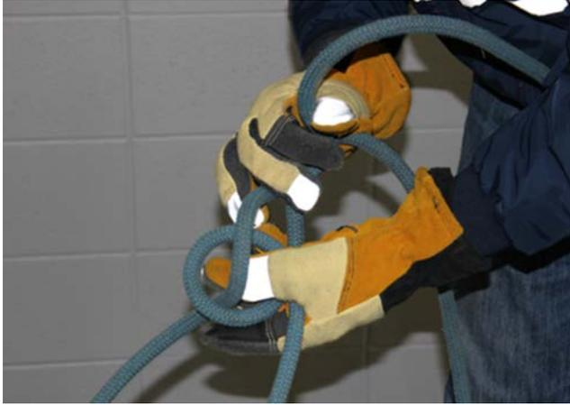
**Figure 2 – Tying knots to test dexterity and tactility**
