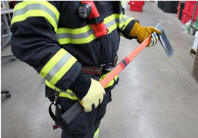
**Figure 4 – Ax used for forcible entry**
