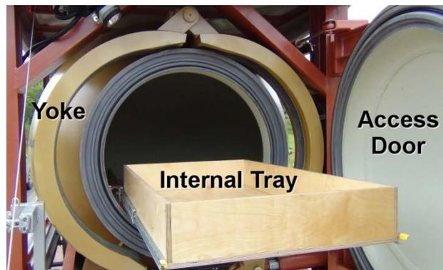
**Figure 2-2. TCV Core Chamber Components**
