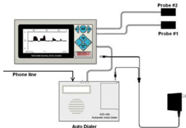
Figure 1. Schematic of Temperature/Humidity Monitor
