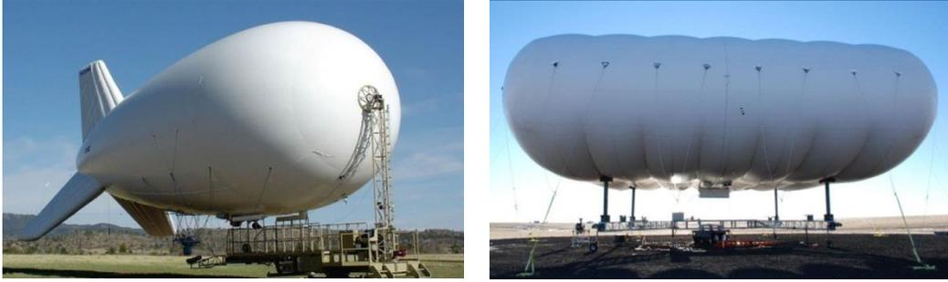
**Figure 2-3. Larger Tethered Aerostat Mooring Stations and Launchers**
