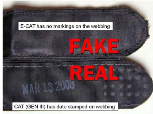
**Figure 2-7. Band Comparison Between a CAT and an E-CAT**
