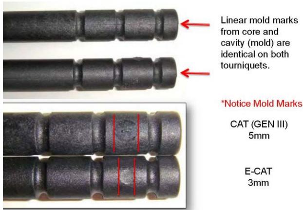
**Figure 2-6. Windlass Comparison Between a CAT and an E-CAT**
