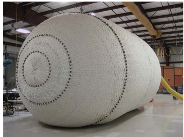
The plug uses special high-strength textiles to withstand the pressures of a flooded tunnel.
