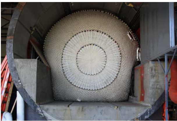
The tunnel plug conforms to the shape of a subway tunnel, as seen in this photo. When deflated, the plug can be stored on the sides of the tunnel without interfering with tunnel operations.
