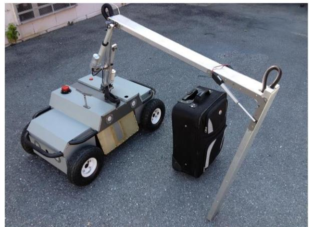
The X-Ray Scanning Rover offers technicians a mobile, high-resolution imaging system that can quickly scan multiple suspicious objects.
