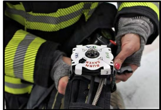
**Figure 3-1 Burn Saver Being Attached to an MSA G1 SCBA Shoulder Strap**
