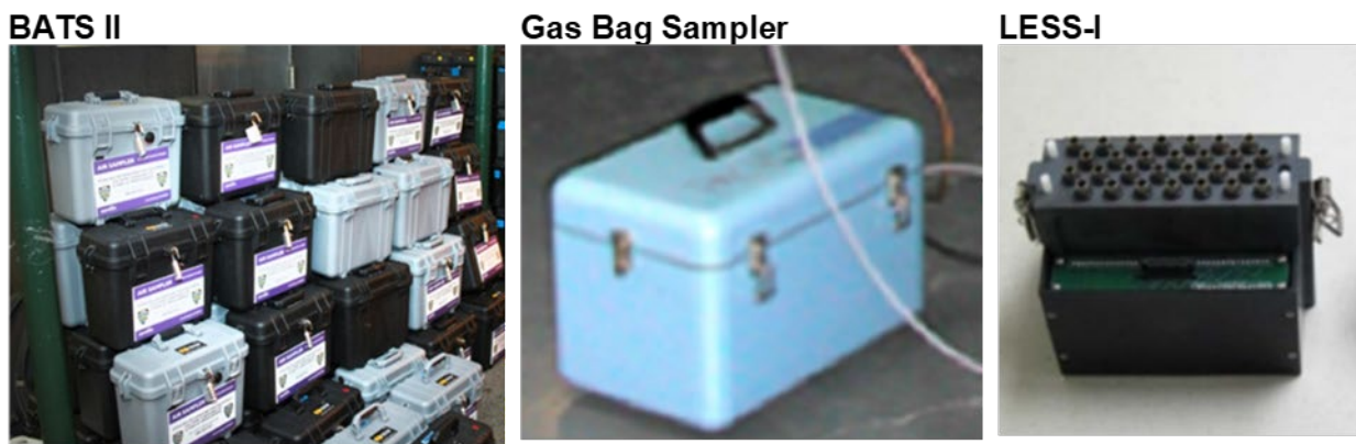
Figure 4. Photographs of gas tracer measurement equipment. The Brookhaven Atmospheric Transport Samplers (BATS II) are shown on the left, and a gas bag sampler is shown in the center, and a LESS-I sequential sorption tube sampler is shown on the right.
