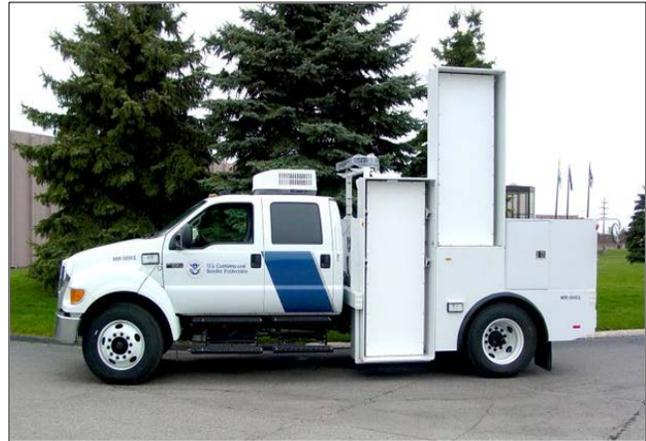
**Figure 2. Mobile Radiation Portal Monitor**
