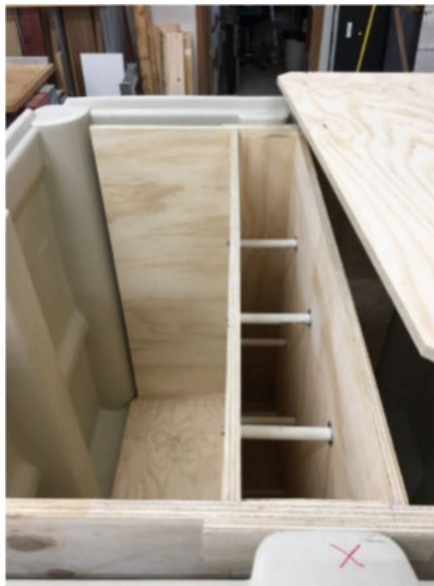
Figure 1: The plywood frame inside the zircon sand container used to hold up a 15 cm slab of sand.
