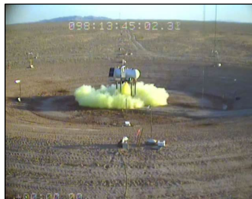
Figure 1-4. Jack Rabbit 1 field test with chlorine release
