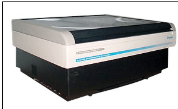
Figure 3-1. The liquid scintillation counter is used to measure radioactivity of a sample material by mixing the active material with a liquid scintillator and counting the resultant photon emissions.
