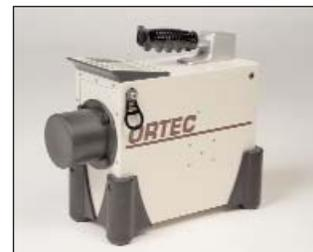
To make this distinction between different radioactive isotopes, it is necessary to perform a spectroscopic analysis using portable gamma spectroscopy systems known as identifiers. Spectroscopic analysis relies on measuring energy of characteristic gamma ray energies emitted by radioactive elements. Collected spectra provide a unique “signature” for identifying the original isotopes. Proper identification of an isotope is important for determining the appropriate response actions.
