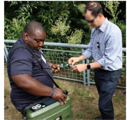
**Figure 4-6 Hapsite ER Pine Needle Vapor Analysis**
