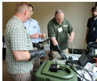
Figure 4-5 Operation of the Hapsite ER with PPE
