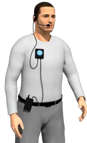
**Figure 1. Key ISC Components Include a Radio, a Headset/Microphone and Push-to-Talk or Voice Activation Device**
