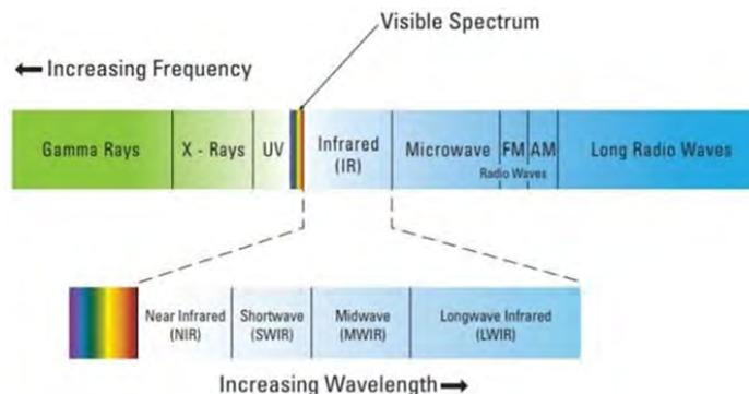
Figure 1. Electromagnetic Spectrum (Image courtesy of FLIR Systems, Inc.)
